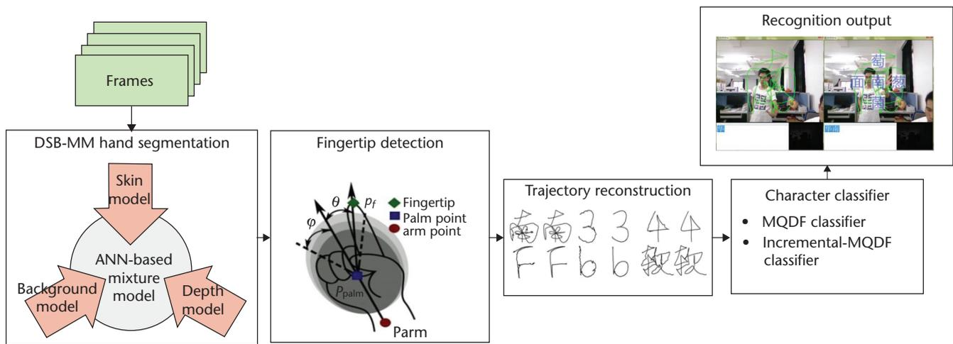
Figure 1. Framework of the finger-writing-in-the-air system.
