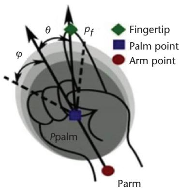
Figure 10. Physical model of a hand for fingertip detection.
