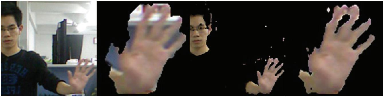
Figure 4. Color depth-model segmentation result. (a) Color image, (b) zoomed-in depth model result, (c) skin-model result, and (d) zoomed-in combination of the depth- and skin-model results.
