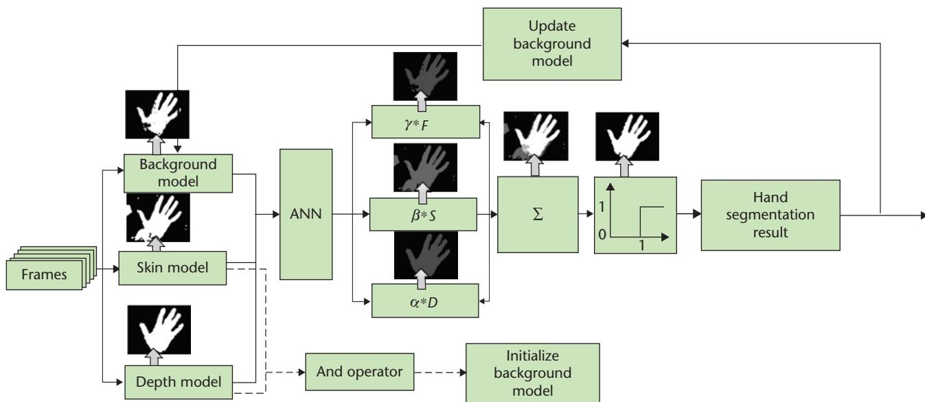
Figure 7. Flowchart of the DSB-MM segmentation algorithm.
