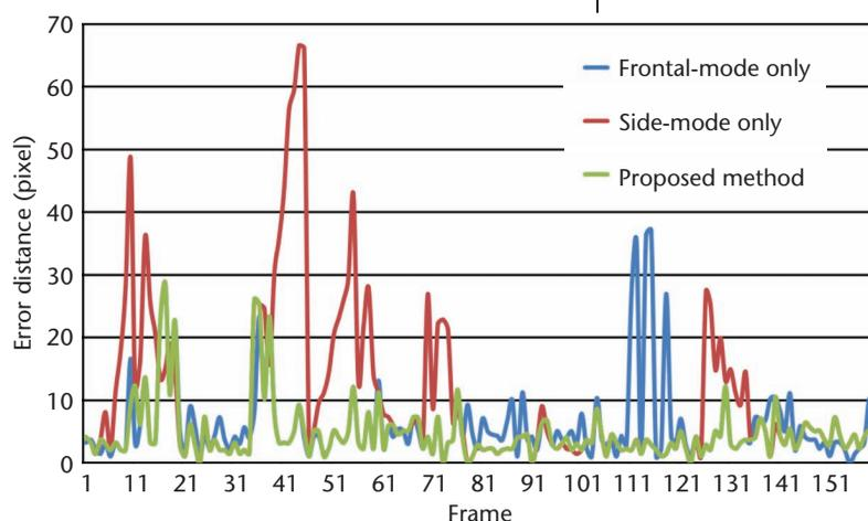
Figure 11. Error distance plots of one video sequence using the frontal-mode-only method, side-mode-only method, and proposed dual-mode switching algorithm.
